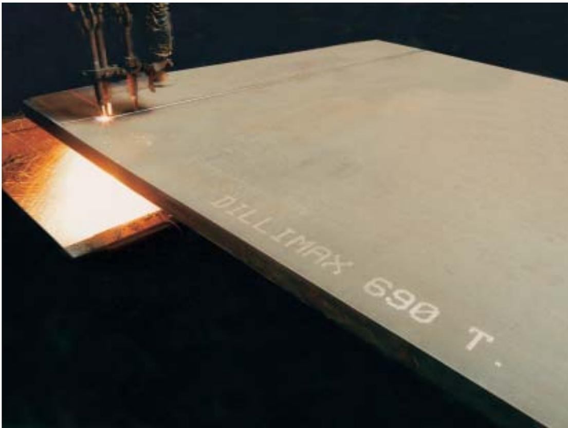
*Figure 9: Oxyacetylene cutting of DILLIMAX 690 T*
