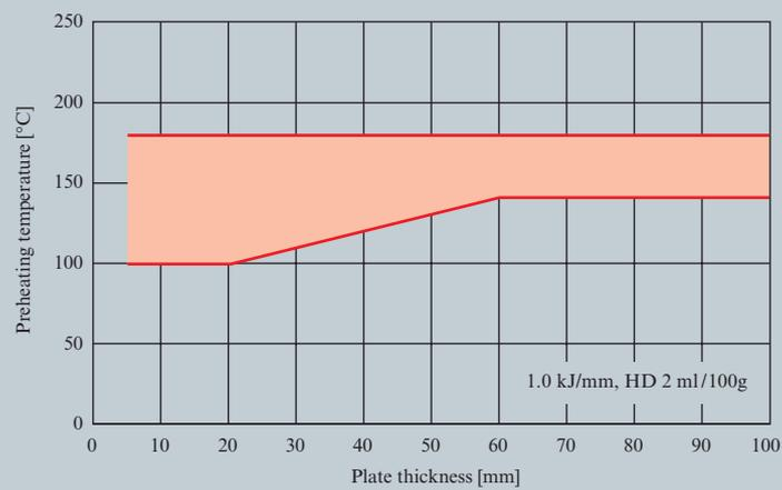
**(b) Gas shielded metal arc welding/fillet weld**
