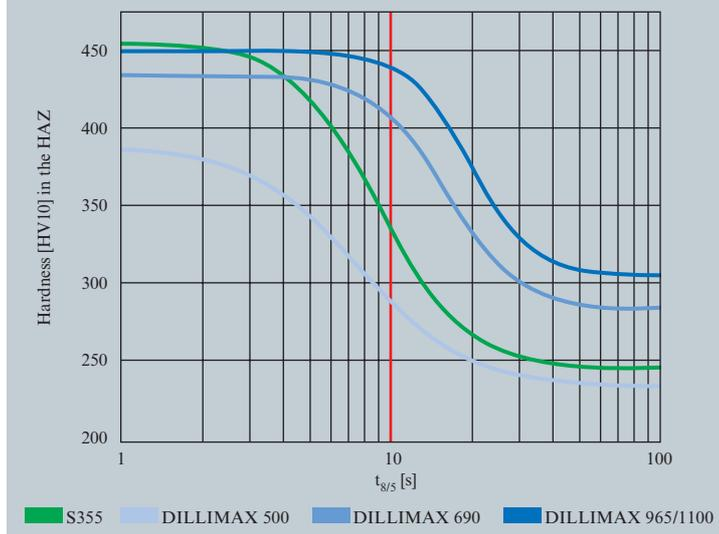
the increased alloy content of base material and fillers. Figure 16 shows typical values
