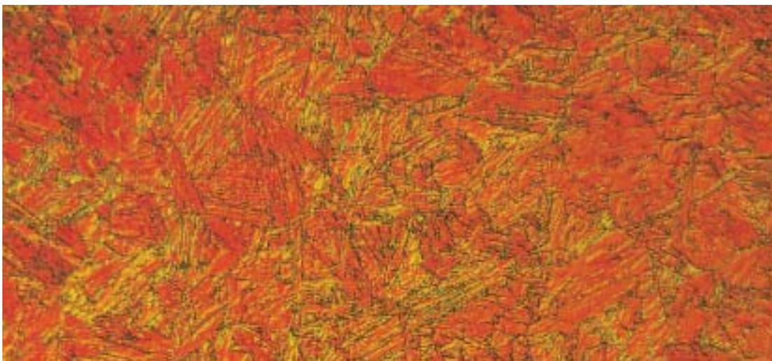
Figure 3: The typical microstructure of DILLIMAX magnified 500 times
