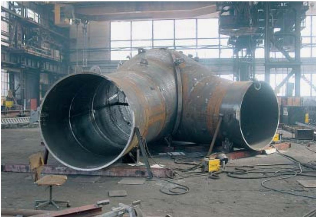
**Figure 6:** Pipes made of DILLIMAX 690 for the penstock linings of the hydropower plant Kárahnjúkar
