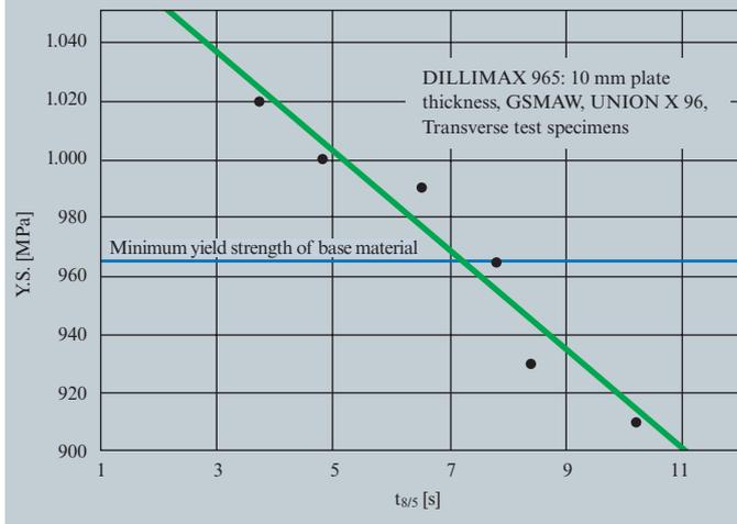
creasing  $t_{8/5}$  time has on the yield strength (Y.S.) of the weld metal.
