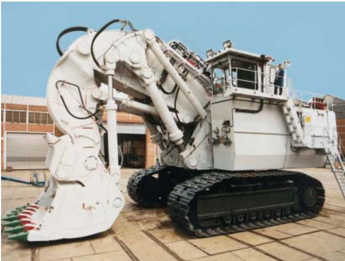
*Figure 4: O&K hydraulic excavator RH 400: Load bearing structural components made of DILLIMAX 690 T
