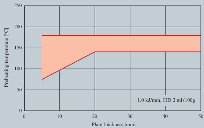
**(b) Gas shielded metal arc welding/fillet weld**
