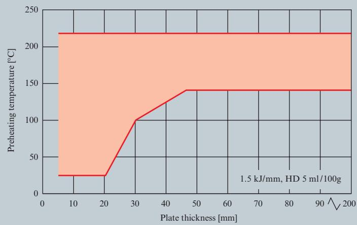
**(b) Gas shielded metal arc welding**
