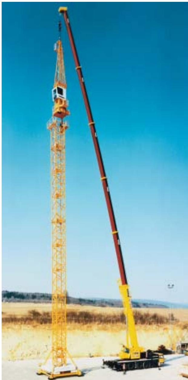
*Figure 20: Mobile crane assembling a tower crane
