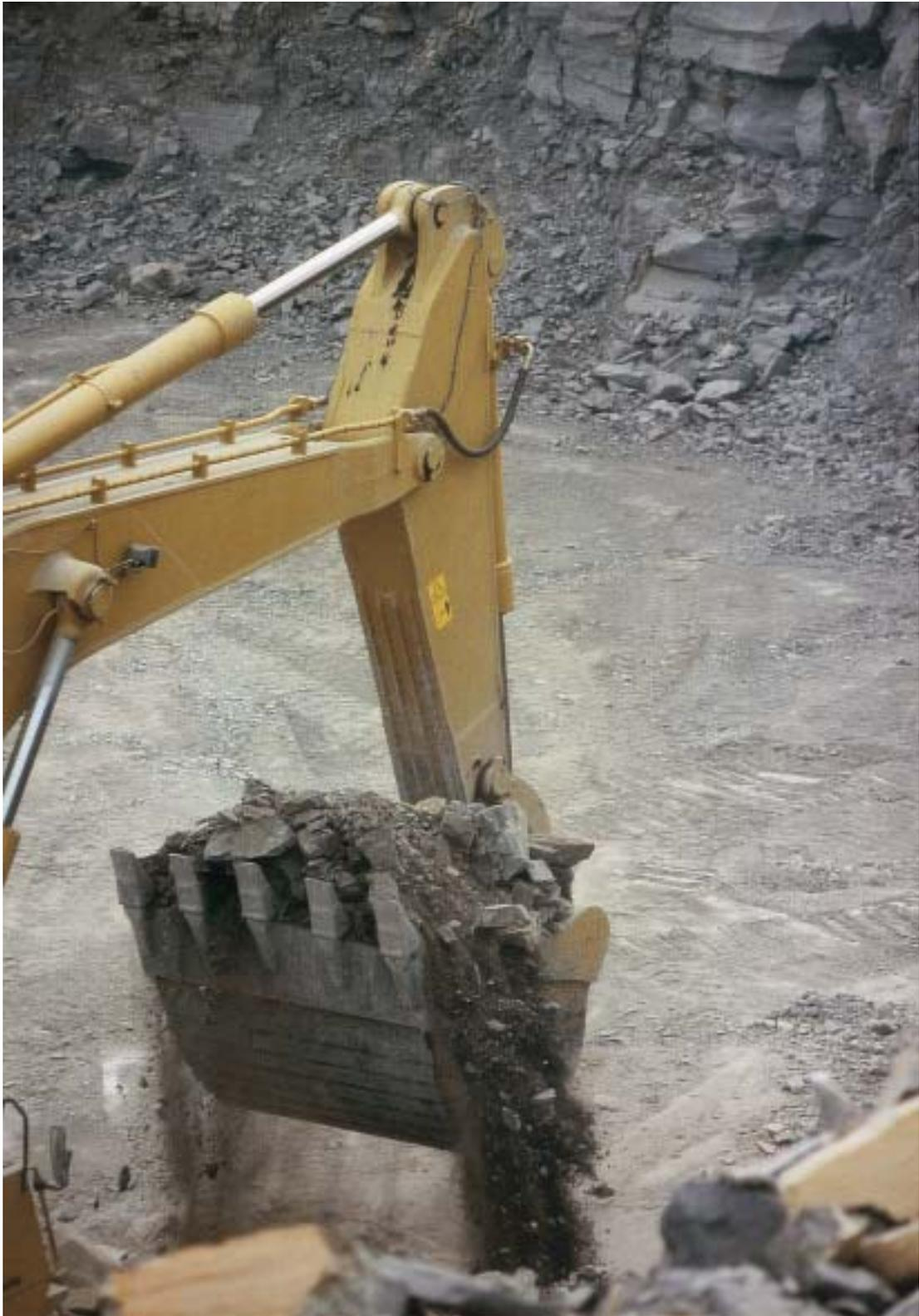
**Figure 1:** Excavator shovel made of DILLIDUR-V steels in the harsh conditions of open-cast mining
