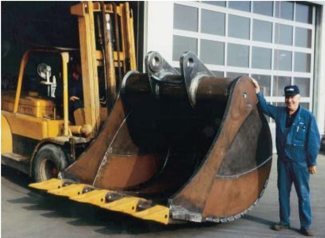
*Figure 20: Welded excavator shovel made of DILLIDUR V plates
