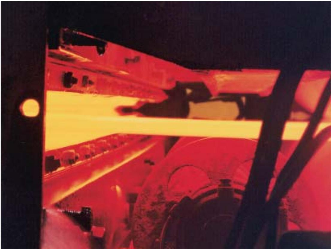
*Figure 5: An austenized DILLIDUR V plate enters the quenching device*
